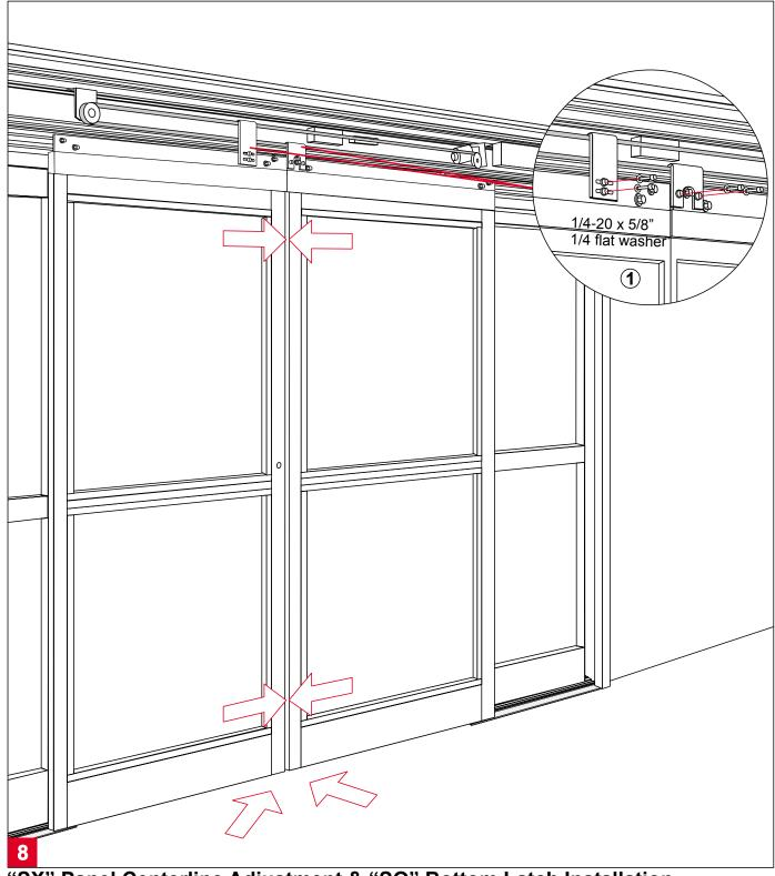
**"SX" Panel Centerline Adjustment & "SO" Bottom Latch Installation** ① With the lower belt bracket securely fastened, and the upper belt bracket in its loose position, the "SX" panels can
