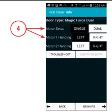
**Step 4**: Setup the Door Type, the **Motor Setup** and the **Motor Handling**.
