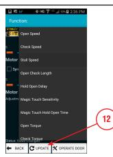
**Step 12**: Configure settings as needed and press **UPDATE** after each settings has been changed. Once completed, press BACK to return to the Main Selection menu. Door must be cycled to Full Open for changes to be stored in permanent memory.
