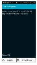
**Step 9**: Put Function switch to **Hold Open** momentarily and then back to **Closed**.
