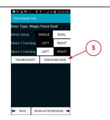
**Step 5**: If additional configuration is needed press **CONFIGURE DOOR**.
