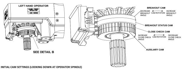
ROTATE BREAKOUT CAMS CLOCKWISE UNTIL RAISED PORTION OF BREAKOUT STATUS CAM JUST CONTACTS SWITCH ROLLER.
