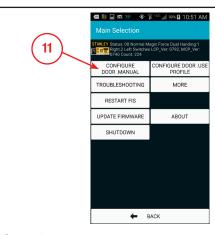
**Step 11**: If the door requires additional changes to be made to the settings, select CONFIGURE DOOR .MANUAL.
