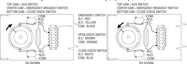
Figure 1. Breakout Status/Breakout Cam Settings (Magic-Swing Operators)
