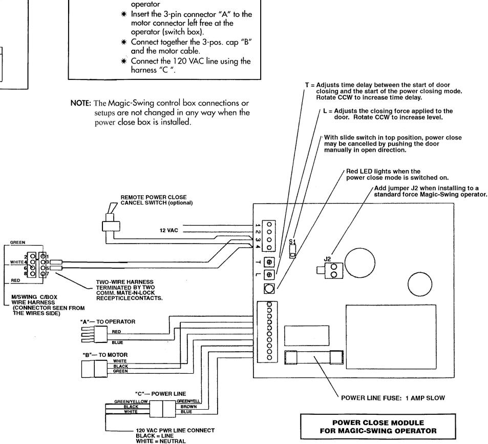
TO INSTALL: \* Disconnect motor cable from the
