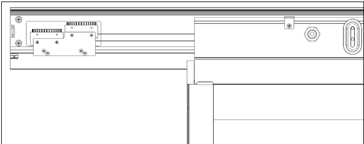
Figure 28: Install the Dual Self-Closer/Damper Kit (Optional)
