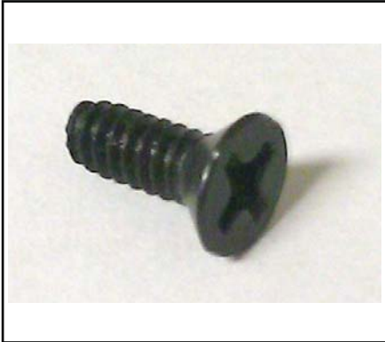
US800734 - DRESS PLATE SCREW FASTENER 6-32x3/8" FL HD THREAD FORMING MS (BLACK OXIDE, BOTTOM LOAD)
